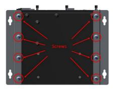
**STEP 2**: Use two screws (Ø3.7 mm, 60 mm in length) per side to attach the MC-7400 to a wall or cabinet.
