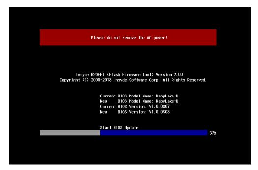
When the upgrade is finished, the computer will automatically reboot. You may check BIOS version on the Main page to confirm the upgrade.
