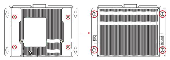
**NOTE** Before tightening the screws into the wall, make sure the screw head and shank size are suitable by inserting the screw into one of the keyhole-shaped apertures of the wall mounting plates.
