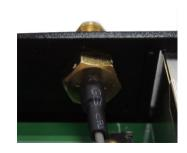
5. Install the connector; place the locking washer first, and then tighten the nut. **Locking Washer**
