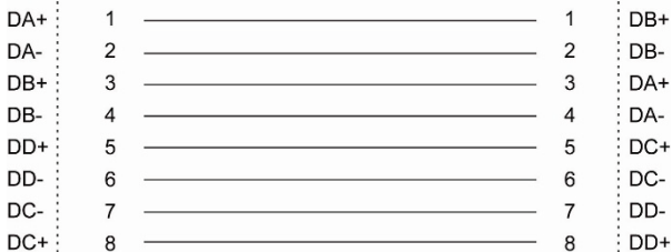
Straight-through Cable Wiring (MDI to MDI-X)
