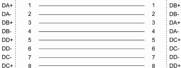
Straight-through Cable Wiring (MDI to MDI-X)
