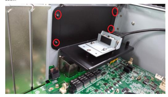
The USB Dongle Kit should be installed as close to the memory socket as possible as shown in the following image:
