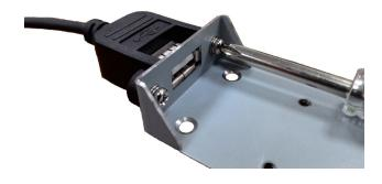
2. Attach the USB Dongle bracket to the tray.
