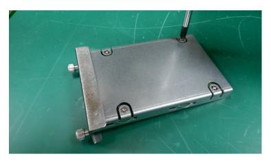
**Step 4:** Insert the SATA Tray into original SATA slot and fasten the screws.
