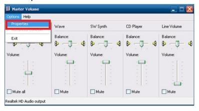
3. Select **Realtek HD Audio Input** from the Mixer device drop-down list, and check **Stereo Mix**. Click **OK** to continue.
