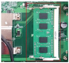
5. There are two latches, one on either side of the memory module. Push the latches outward to release the memory module. The memory module automatically pops out. Gently remove the memory module.
