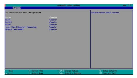
**RAID 0** is a simple striping of information across two drives. It offers marginal improvements in access times for substantial sacrifices in system reliability.
