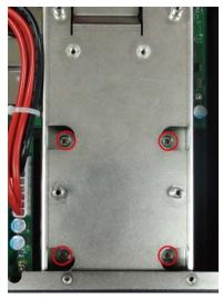
4. When finished, remove the storage tray cover to expose the memory module.
