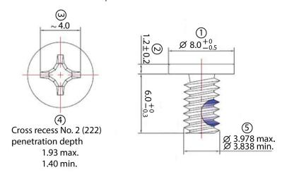
To mount a BXP-C100 computer to a wall or cabinet, use two screws on each side for the mounting brackets as shown in the illustration.
