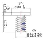
To mount a BXP computer to a wall or cabinet, use two screws on each side for the mounting brackets as shown in the illustration.
