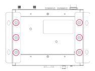
The six screws for the mounting brackets are included in the product package. Refer to the following illustrations for detailed specifications.
