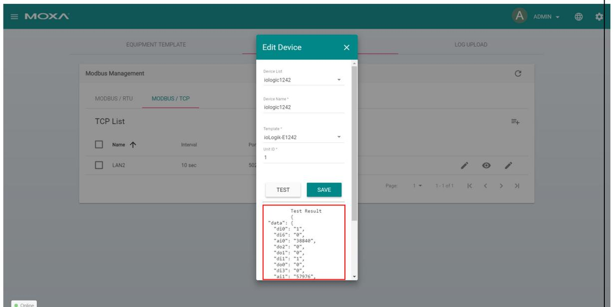
If the test result shows no errors, the Modbus device is set up correctly.
