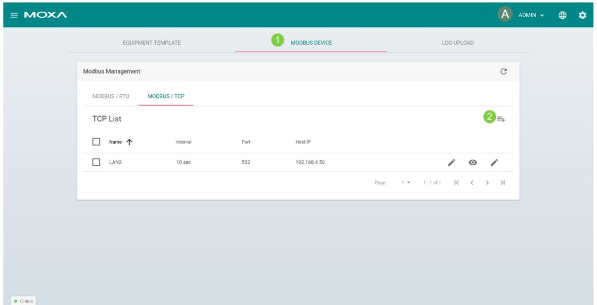
In this example, the iLogik-E1242 Modbus device is set up with 192.168.4.50 as the IP address. The query interval for the device is set to 2000 milliseconds.
