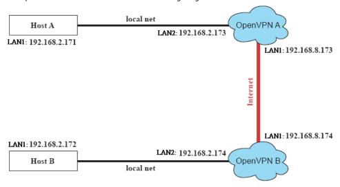
2. The configuration procedure is almost the same as for the previous example. The only difference is that you will need to comment out the parameter "up" in "/etc/openvpn/tap0-br.conf" and "/etc/openvpn/tap0-br.conf".
