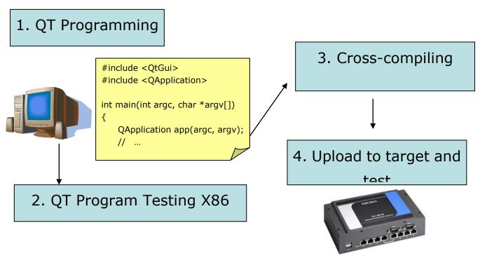
Write the QT program to run the in thetarget environment. A basic QT program is shown below.
