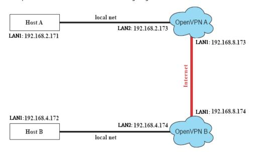
2. On machine OpenVPN A, modify the remote address in the configuration file, /etc/openvpn/tun.conf.
