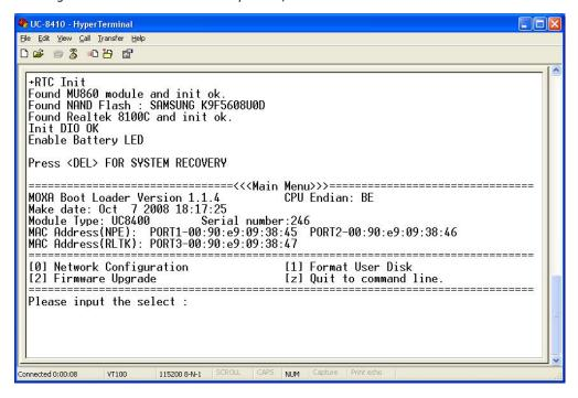
1. In the boot loader utility, select **[0] Network Configuration**, and then **[0] Change IP Setting** to configure IP addresses.
