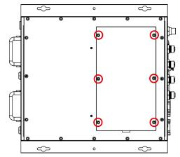
2. Install the hard disk onto the internal storage kit. Connect the cable and connector.
