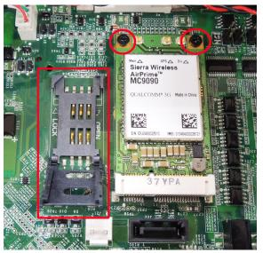
3. Insert the SIM card in the holder by first dropping the holder into place (flush with the board), and then locking it down by sliding it into place.
