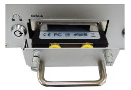
When finished, turn the key clockwise to activate the lock and tighten the thumbscrews. Use the same method to install a hard disk in second storage tray.
