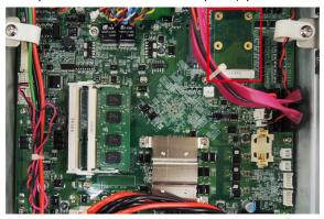
2. Install the module into the socket. Fasten two screws on one end of the module. In addition, pull up the SIM card holder beside the socket.
