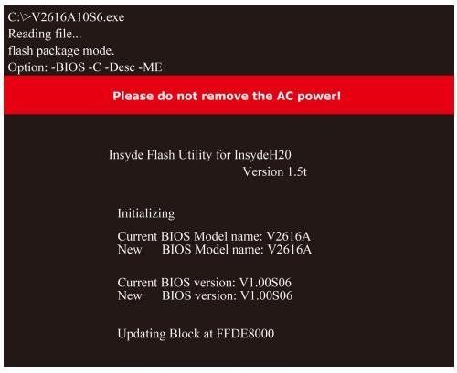
6. When the upgrade is finished, the computer will automatically reboot. You may check the BIOS version on Main page of the BIOS Setup
