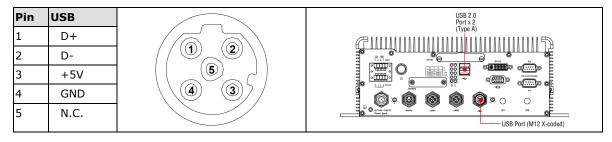
**NOTE** This is the pin assignment for the computer-side USB ports on the V2616A shell. If you are wiring peripheral-side connectors for a USB cable, you will need to **mirror** the pin assignment.
