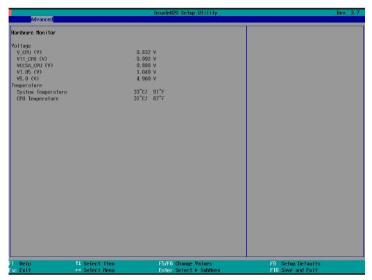
Note that the voltage values are different for different models. The temperature readings shown on the screen are within  $\pm 5\%$  of the actual readings. However, the temperature readings are only valid when the ambient temperature is above 0°C.
