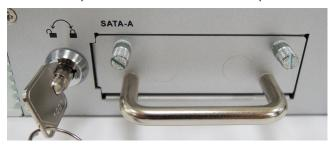
3. Pull out the faceplate by unscrewing the thumbscrews in the upper corners, and then remove the plate. Fasten the storage drive to the faceplate flange as shown below, using the two flathead screws that were shipped with your V2616A.
