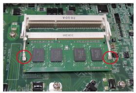
5. After removing the memory card, install the new module by gently but firmly inserting it into the RAM slot. Before securing the card in place, be sure you have aligned the indentations on each side of the card with the mechanical locks that will hold it in place (shown at right, in the red circles). Once the card is properly aligned, gently push the card down, until it locks in place. You should hear an audible click; before continuing, make sure the latches are firmly in place.
