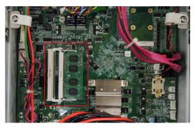
Carefully remove the module by pushing the latches on both sides of the module, freeing it to be removed.
