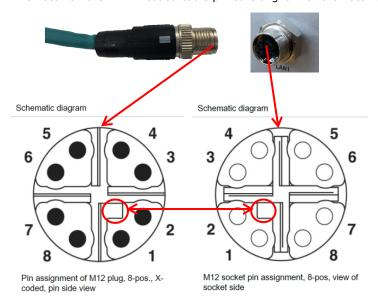
3. Connect the M12 X-coded cable to the port.
