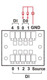
**NOTE** If you are using wet contacts, you must connect **source** to power. In addition, both DI and DO can only be wired as **sink** type**s**
