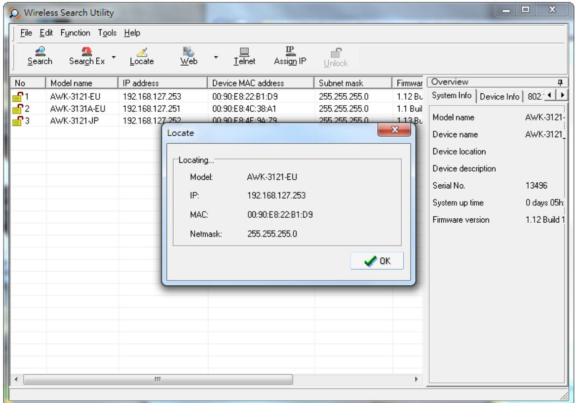
Make sure your AWK is **unlocked** before using the search utility function buttons (Locate, Assign IP, etc.). The AWK will unlock automatically if the password is set to the default. Otherwise you must enter the new password manually.
