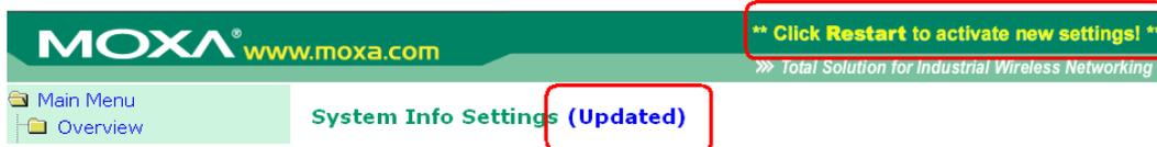
To activate the changes click **Restart** and then **Save and Restart** after you change the settings. About 30 seconds are needed for the AWK-3121 to complete the reboot procedure.
