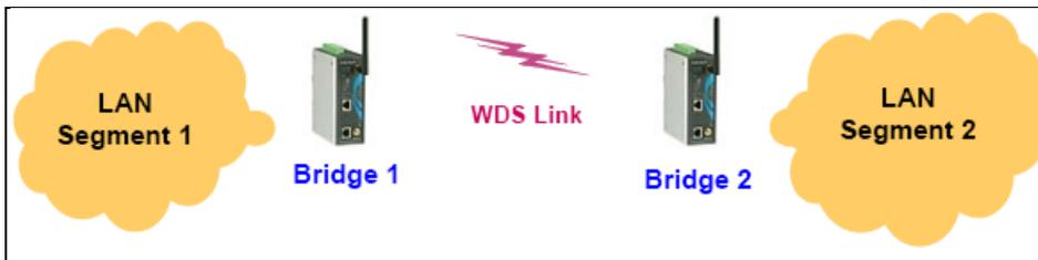
It is a good idea to plan your wireless network by drawing a diagram so that you know how each AWK-3121 is connected to other peer APs or wireless bridges by WDS, and how bridges are connected to other peer bridges by WDS. See the following figure for an example of a network-planning diagram.
