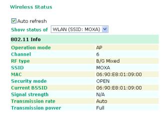
**NOTE** The **802.11 info** that is displayed may be different for different operation modes. For example, "Current BSSID" is not available in Client mode, and "Signal strength" is not available in AP mode.
