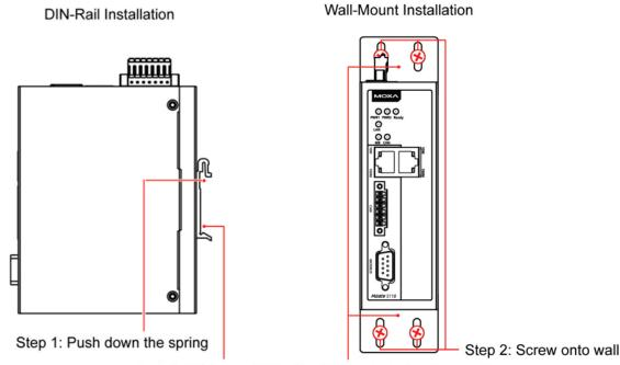
Step 2: Click onto DIN rail Step 1: Install wall-mount kit
