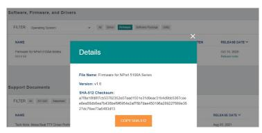
• When a user wants to upgrade the firmware of the NPort 5000 Series, please download the firmware from the website first. Then log in to HTTP/HTTPS console and select **Upgrade Firmware**. Click the **Choose File** button to select the proper firmware and click **Submit** to upgrade the firmware.
