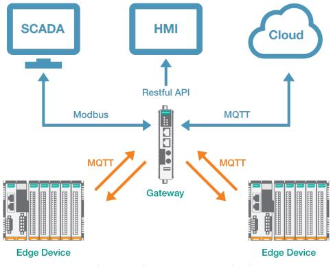
Figure 8. Architecture for connecting to a local gateway
