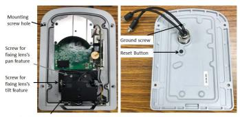
Calibration for tuning lens's vertical (-5 to  $10^{\circ}$  ) and horizontal (+/-  $5^{\circ}$  ) position
