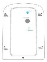
**NOTE** The recommended torque of the top cover is 12 kg-cm and 25 kg-cm for mounting the camera on the train.
